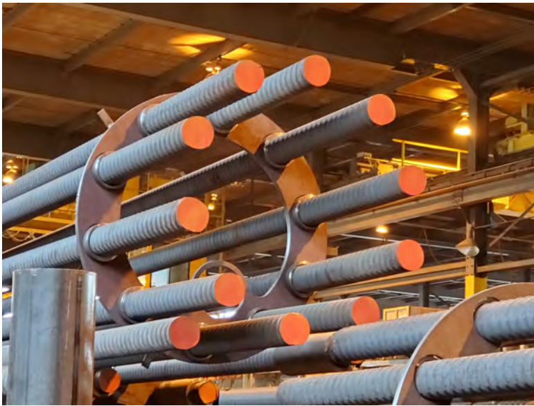
Above: Prefabricated Caisson cages in SSSI Warehouse
